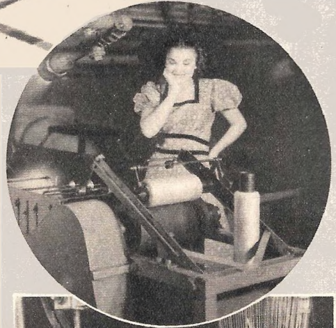
Below: Fascinating to watch is this "staple process" of forming glass threads. The molten glass is blown down past the drying flame at the edge of the picture, and forms almost out of thin air as fine white threads, which are taken up on the spools.
