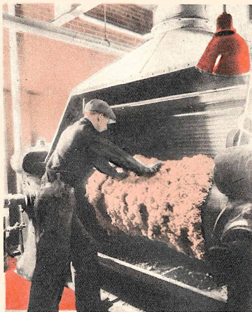
Plasticizing and drying neoprene. Apparatus unlike anything the chemical industry ever before knew made it possible for chemists to produce a rubber substitute that excels Nature's product in its adaptability.
