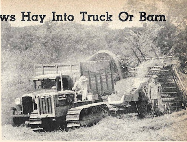
Cutting hay into small bits, enabling a large quantity to be stored in a small space, this machine also loads hay into trucks or barn mows by blowing it through a long pipe.
