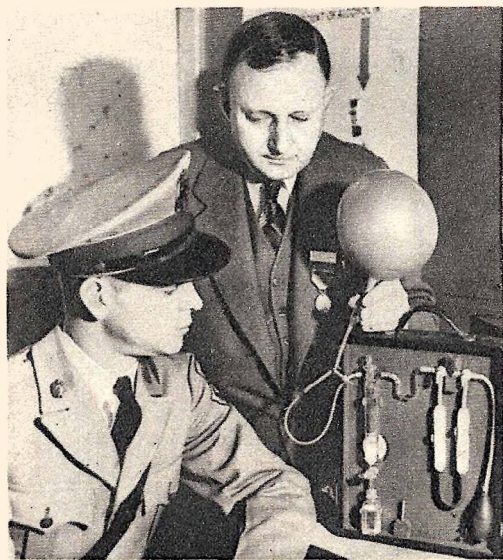
Professor R. N. Harger shows a Missouri trooper his new device for checking amount of alcohol in autoist's breath.
