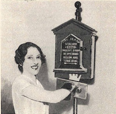
Demonstrated above is a new fire signal box that locks the hand of alarm sender until released by a policeman or fireman with a key, thus deterring the sending of false alarms.
