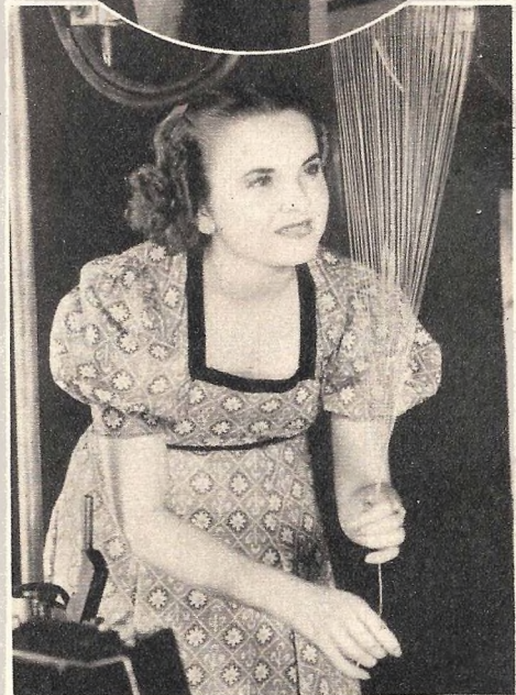
In the "continuous filament" process, 102 fine strands of glass, formed by tiny holes through which the molten glass passes, are formed into a single thread. They have been greatly retouched in this picture, actually they are hardly visible to the eye.
