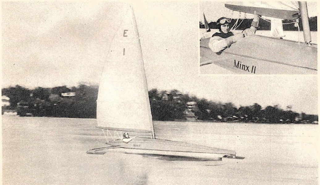
Designed for Class E racing, this ice boat features many improvements. Close-up shows pivot joint of free-rotation mast.
