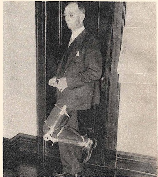
Criminals can walk, but not run, when wearing the "legcuff" demonstrated above. Device locks if running is attempted.
