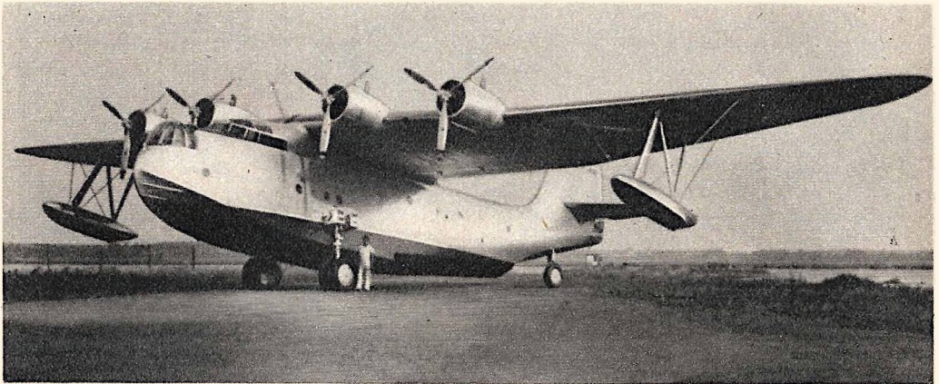
Four engines of 1,050 horsepower each are required to power this huge Sikorsky flying boat. Plane has three gun turrets.
