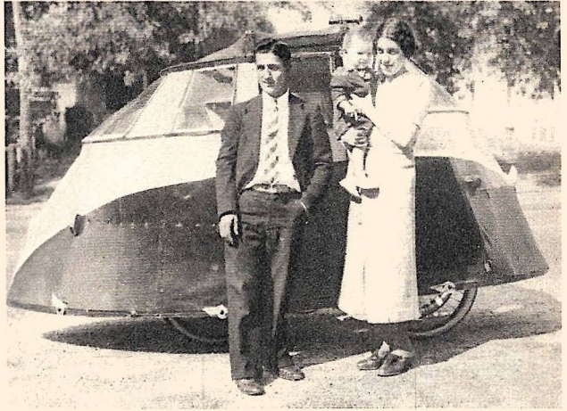
The A. Martin family of Dracutt, Mass., uses this "Cyclemobile" for trips to nearby towns. Vehicle consists of two bicycles joined together and covered with a canvas hood.
